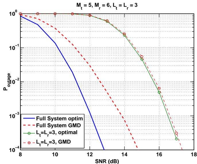
Fig. 6. The outage probability of GMD and optimal system with and without AS.  $M_t = 5$ ,  $M_r = 6$ ,  $L_r = L_t = 3$ , and target rate  $R = 14$  bps/Hz.
