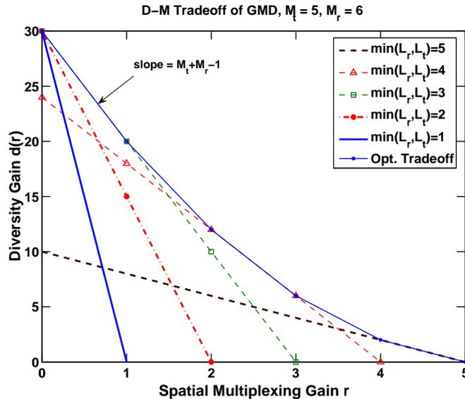
Fig. 2. The D-M tradeoff of the GMD scheme applied to a RF-chain limited system with AS vs. the optimal D-M tradeoffs of full MIMO system
