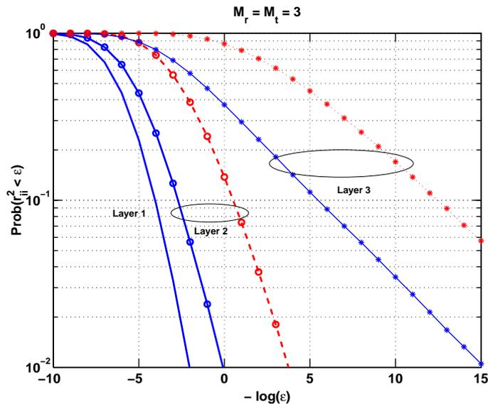
Fig. 4. The outage probabilities of the layers. The solid lines stand for the outage probability  $\mathbb{P}(r_{ii,\max}^2 < \epsilon)$  and the marked dot lines represent  $\mathbb{P}(r_{ii}^2 < \epsilon)$ .
