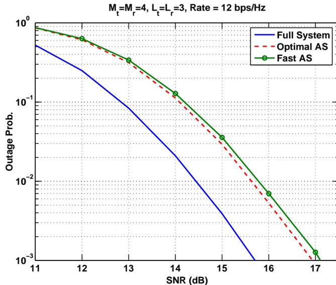
Fig. 3. Outage probabilities of the full MIMO system and the pruned system obtained via optimal AS and proposed fast AS algorithm
