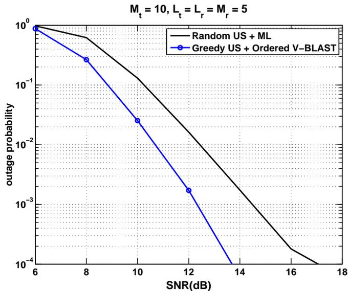
Fig. 5. The outage probabilities of MAC with ML receiver and random user selection (US) versus the ordered V-BLAST scheme combined with greedy user US. The sum rate is 10 bps/Hz and is equally distributed among five users.
